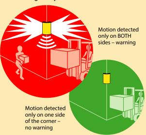
The Collision Sentry only sends a warning when it senses objects moving in both of its detection zones.
