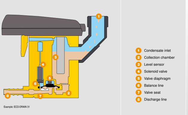
The condensate passes through the condensate inlet (1) into the collection chamber (2). The level sensor (3) detects the presence of condensate and sends a signal to the drain's control system when a preset condensate level is reached. This opens the solenoid valve (4) and also therefore the pressure balance line (6). The resulting pressure compensation causes the valve diaphragm (5) to open. The condensate flows from the collector through discharge line (8) from
