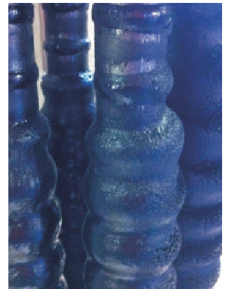
Ferritic particles on magnetic filter rods
