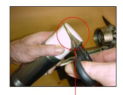
INSERT NEW CARTRIDGE WITH THE END 'SEALED FACING UP, CUT AND SCREW
