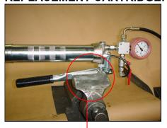
PLACE IN THE VICE PUMP, LOOSEN THE TANK AND REMOVE CARTRIDGE OUT
