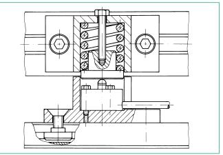
Overload of the load cell is impossible due to a suitable spring. When the units are locked the spring will transfer not more load to the cell than the measuring range can cope with.
