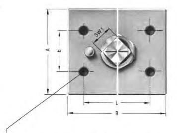
Mounting pad holes for actuator brackets are optional.
