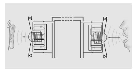
In principle only two capsules are needed to build a dynamic telephone system. An electric power supply is not necessary. The two capsules must be connected by any two-wire cable. Used as a microphone, the dynamic capsule generates a relatively high voltage from a low sound pressure. This voltage suffices to generate a sufficiently high sound pressure at the other capsule used as loudspeaker.
