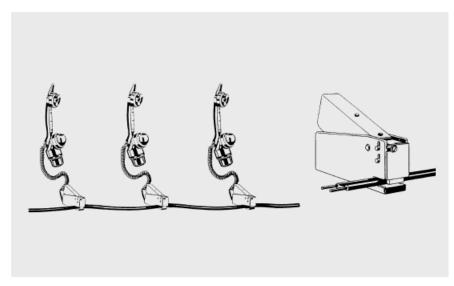
**3.** With firmly installed cable, for plug-connected hand telephones and / or permanently installed wall telephones
