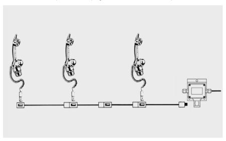
2. With movable telephone cable, with "prick pincers" – the quick connection from any part of the cable
